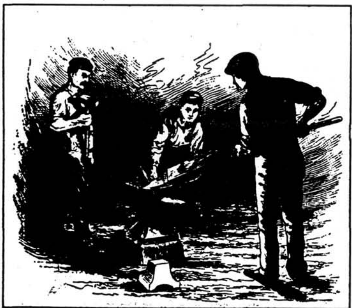
Figure 4 -- Finishing the horn by hand.
