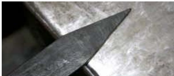
Fig. 21. Place just the set-up flat on the anvil face.
