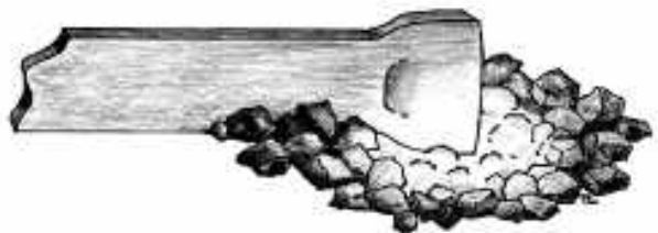
Fig. 13. Half to be worked placed edge down in the fire.
