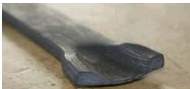
Fig. 10. Top of the bar showing peened middle trough.
