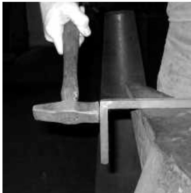
7. When trueing the angle to 90 degrees, keep the short leg away from the anvil as shown here. Doing so will keep you from reducing the cross-section of the bar beneath the parent stock size.
