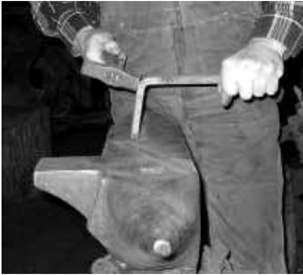
3. Stand at the heel of the anvil to forge this form.
