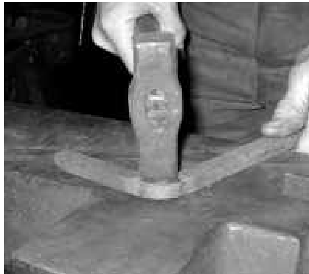
2. Position the hammer as shown when cross-peening the corner. Be mindful that you do not reduce the cross-section smaller than that of the parent stock.
