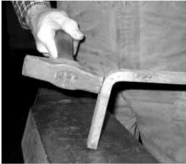
5. Horizontal blow—Note the position of the hammer and the short leg.
